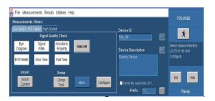
**4.** Select Measurement > Configure and set up the application in the Configure and Source tabs.
